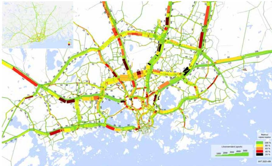
Fig. 3. Bottlenecks in the morning peak in the Helsinki region in 2025 in the HLJ 2015 base alternative (VE0). Sections of road with speed less than 60% of free-flow conditions. In the picture, the colors depict the sections of road as follows: orange = prone to congestion, red = congested, black = highly prone to congestion
