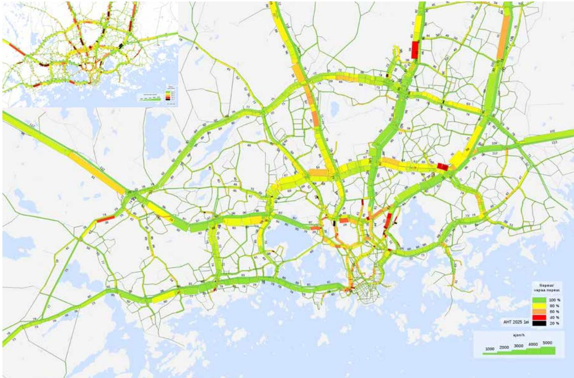
Fig. 6. Bottlenecks in the Helsinki region in the morning peak in 2025 have been depicted using the HLJ 2015 gate zone pricing model (VE1). Sections of road where the speed is less than 60% of the free-flow conditions. In the picture, the colors depict the sections of road as follows:
