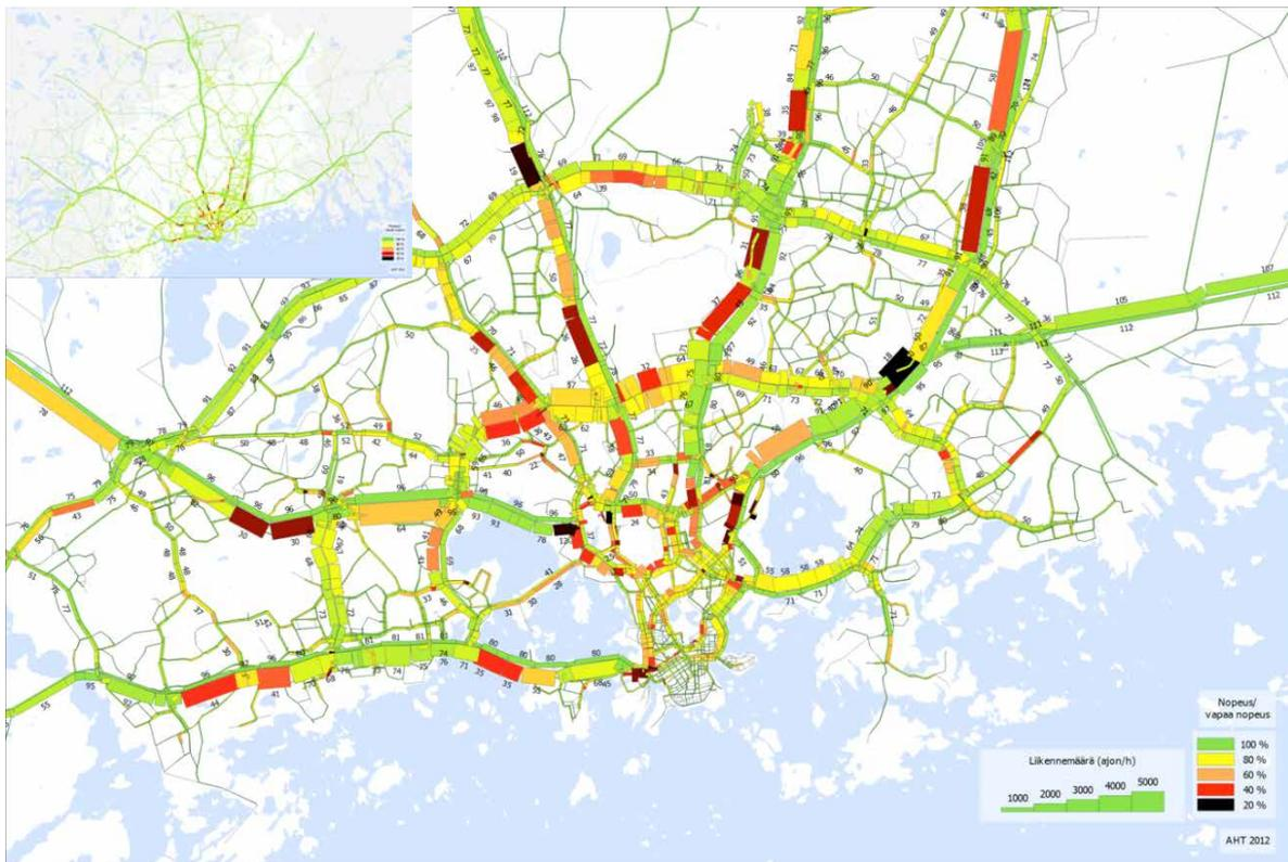
Fig. 1. Bottlenecks in the Helsinki region in the morning peak in 2012. Sections of road where the speed is less than 60% of the free-flow conditions. In the picture, the colors depict the sections of road as follows: orange = prone to congestion, red = congested, black = highly prone to congestion
